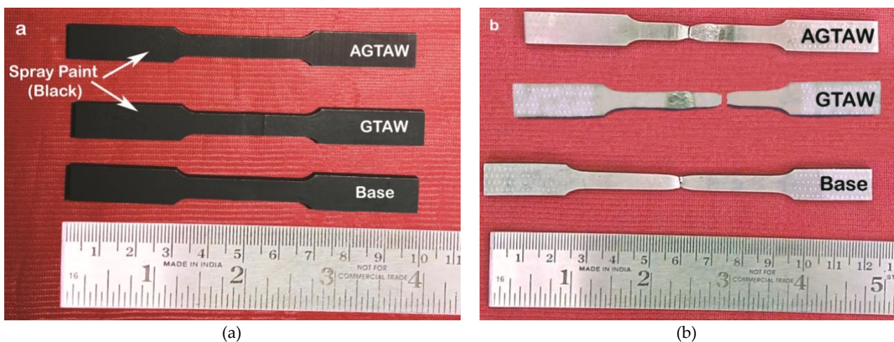
Fig. 2. Tensile Sample a) before the test b) after the test
