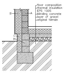
Fig. 1. Establishment with thermal insulation of basis and external wall A - Ytong P2-400, B - expanded polystyrene EPS 70F, C - extruded polystyrene Styrodur 2800C, H - form block DT30
