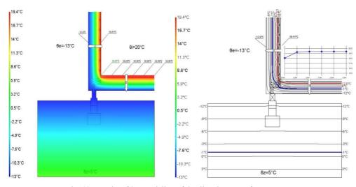
Fig. 10. Results of 2D modeling of detail and course of temperature
