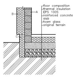
Fig. 5. Establishment on brash of foam glass
