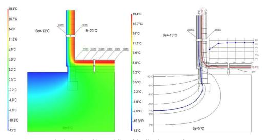
Fig. 4. Results of 2D modeling of detail and course of temperature
