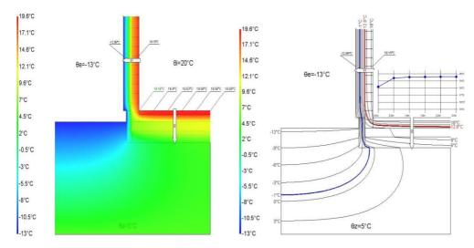
Fig. 6. Results of 2D modeling of detail and course of temperature
