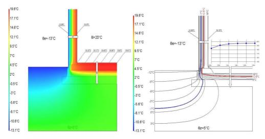
Fig. 8. Results of 2D modeling of detail and course of temperature
