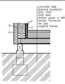
Fig. 9. Establishment on pilots D - mineral wool Isover TF profi, E - OSB slab, F - mineral wool Isover Unirol profi, G - gypsum plaster slab
