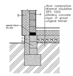
Fig. 3. Establishment with special block, with plinth insulation A - Ytong P2-400, B - expanded polystyrene EPS 70F, C - extruded polystyrene Styrodur 2800C, H - form block DT30
