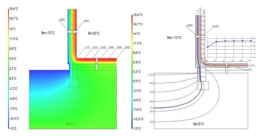
Fig. 2. Results of 2D modeling of detail and course of temperature
