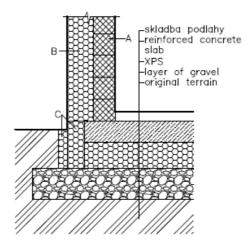
Fig. 7. Establishment on tub of extruded polystyrene boards A - Ytong P2-400, B - expanded polystyrene EPS 70F, C - extruded polystyrene Styrodur 2800C
