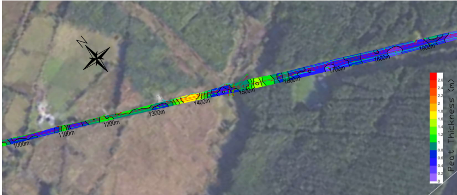
Fig. 16. Aerial imagery with overlaid layer of Peat Thickness created in “Surfer” based on GPR Investigation data
