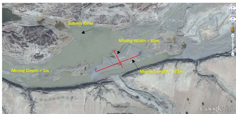
Fig. 6. Geometrical dimensions of the sedimentary deposit considered for material mining along the Zohreh River; source: own elaboration
