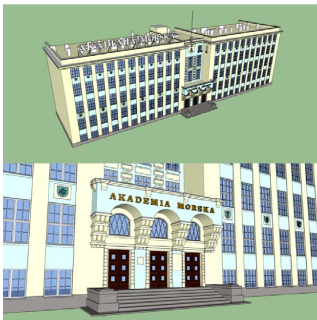
Figure 1. 3D Model of the main building of Gdynia Maritime University developed with the use of photogrammetric techniques [source: own study]
