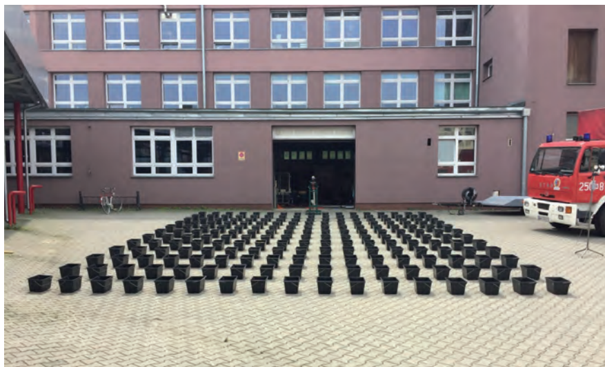
Fig. 6. The view of the test stand and the real special regular grid of measuring containers before one of the experiments
