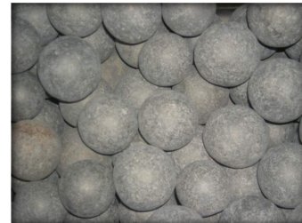
Fig. 2. Cast iron spheres, constituting additional grinding-crushing elements of the prototype reclaimer
