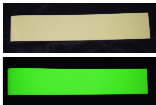
Figure 1. Photoluminescent material strip view (top) and lighting effect of the strip after main lighting goes out (bottom)
