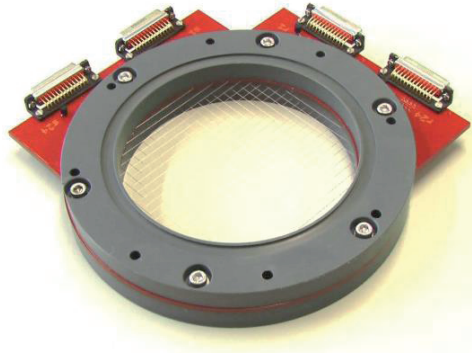
Fig. 4. Photograph of the applied wire-mesh sensor with an ID of 0.15 m.
