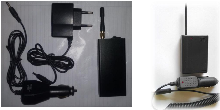
Fig. 2. The jamming device made by Spy Electronics LTD (left) and GX-40B made by TTS (right) [authors' photos]
