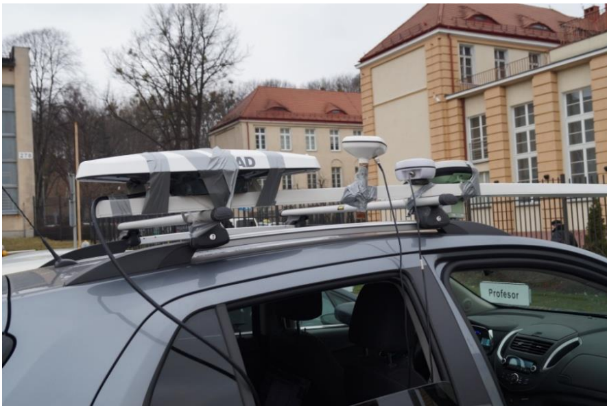
Fig. 4. The way the antennas were fitted [authors' photo]
