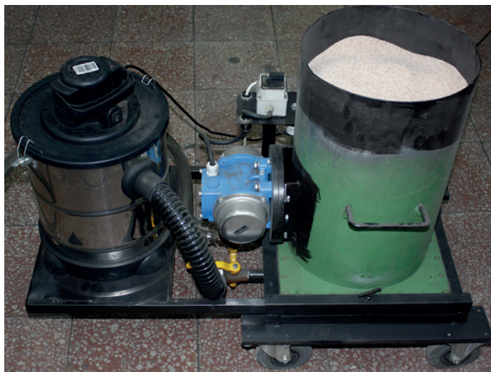
Fig. 8. Laboratory stand for the full-mould technology investigations
