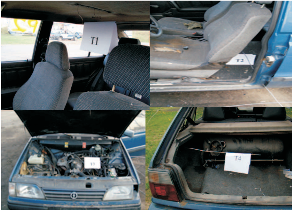
Fig. 2. Location of the thermocouple in a car
