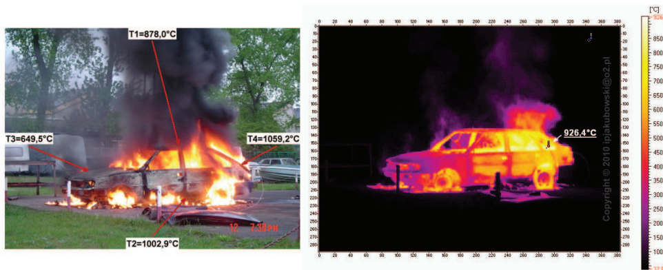
Fig. 8. The photo and the thermagram of burning car
