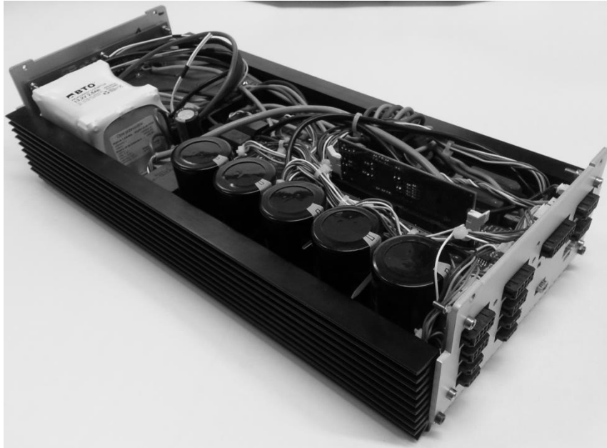
Fig. 3.3. Photograph of the scaled down PRT vehicle propulsion and power supply module
