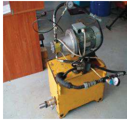
Fig. 25. Testing stand for gear pumps
