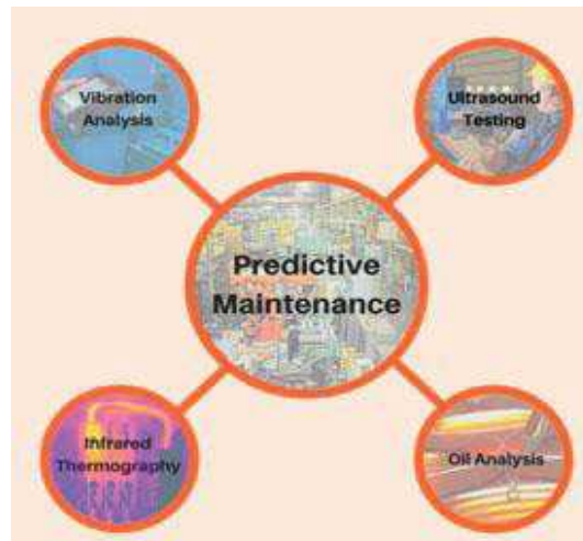
Fig. 2. The most common predictive maintenance methods [4]
