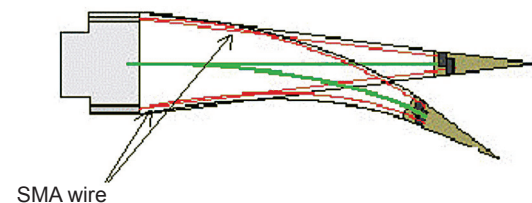
Fig. 7. Schematic of layout of wires comprising a shape memory material [7]
