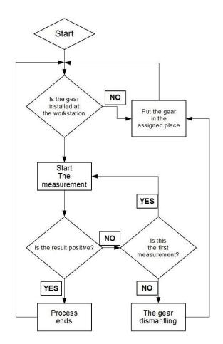
Fig. 4. The algorithm to control the validation workstation for the gears installation [9]
