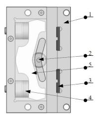
Fig. 1. Diagram of CHP2000 type progressive gears: 1 – a body, 2 – a braking roller, 3 – a braking plate, 4 – Belleville springs, 5 – a cam [5]
