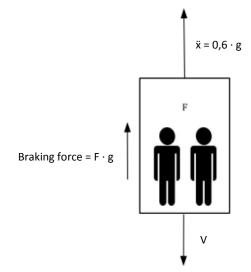
Fig. 3. The relationship between the speed, delay vectors and the braking force [3]
