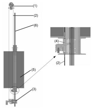
Fig. 2. The location of the braking system subassys of the friction gear, 1 – the speed limiter, 2 – the speed limiter line, 3 – a tensioning weight, 4 – a gear with a lever assy, 5 – the cabin with a frame, 6 - a guide [6]
