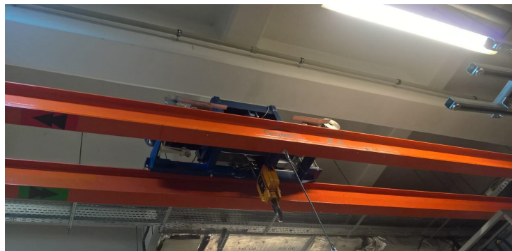
Fig. 1. The double-girder overhead traveling crane with hoisting capacity 1000 kg
