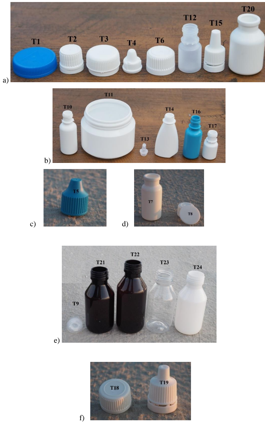
Fig. 1. The materials described in Table 2: a) HDPE, b) LDPE, c) PS, d) PE, e) PE, f) PP
