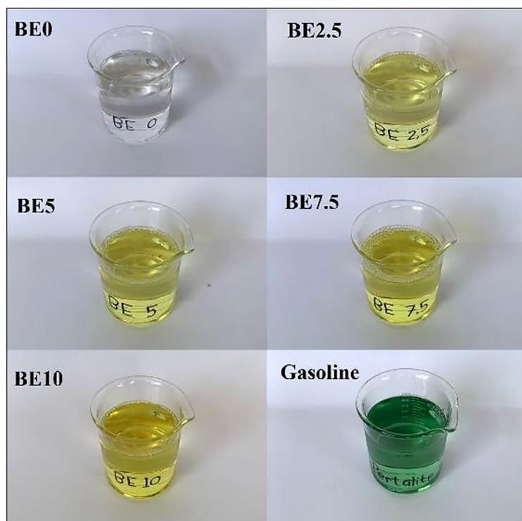
**Figure 1.** Appearance of BE0-BE10 fuel and commercial fuel as a comparison
