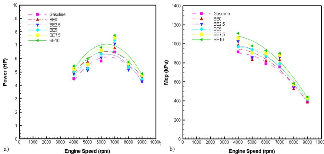
Figure 4. (a) Power variation with engine speed (b) effective pressure variation with engine speed
