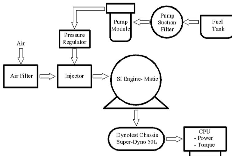
**Figure 2.** Engine performance testing scheme
