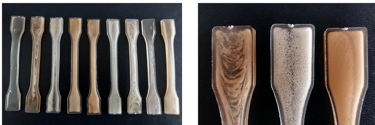
Fig. 3. Porous PVC injection molded parts with an ingot and a fragment of the molded part with a visible porous structure
