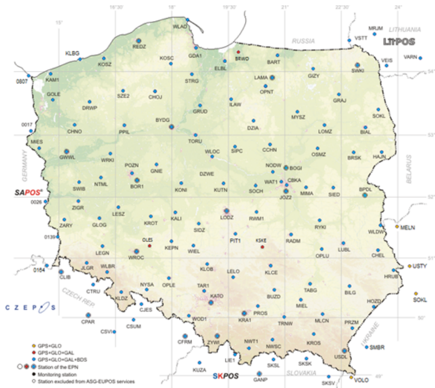
Fig. 6. Reference stations of the ASG-EUPOS system (as of February 2023, www.aseupos.pl )
