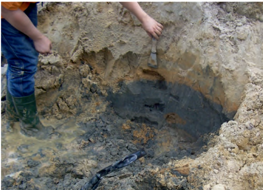
Fig. 6. Geological section on the East Volodymyrets deposit, Rivne region. The productive horizon of the Mezhyhirsk suite, i.e. dark gray quartz-glaucanite sands, is at the bottom of the exploratory pit. Photo by O. Remezova
