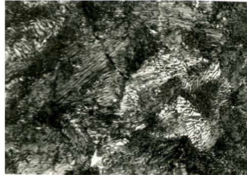
Fig. 12 Microstructure of pressure steel cast made of steel 11373 as viewed through the optical microscope, x1000 ηm
