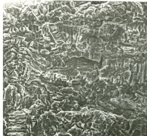
Fig. 13 Microstructure of pressure steel cast made of steel 11373 as viewed through the electron microscope, x1000 ηm
