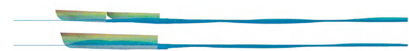
Fig. 21. Wave side view comparison of two hulls at different F_r
