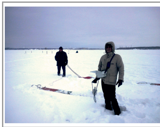
Fig. 5. Loza-N GPR survey around frozen ice-hole in lake Chebarkul.
