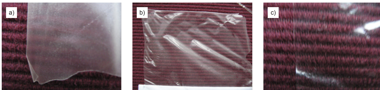
Figure 2. Images of cellulose film made from 5.0 wt% cotton linters in IL, where a - RCF 2A (coagulation bath - demineralised water); b - RCF 2B (coagulation bath - EtOH); c - RCF 3A (coagulation bath - EtOH, second bath - EtOH).
