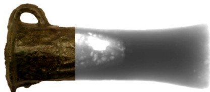
Fig. 9. X-ray image of axe No. NG15 together with the view of part of the artefact with visible defects
