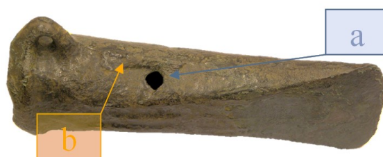
Fig. 6. Axe (No. NG7) with remained elements of the gating system and casting defects: incomplete filling - misrun (a) and flashes along the line joining the mould (b)
