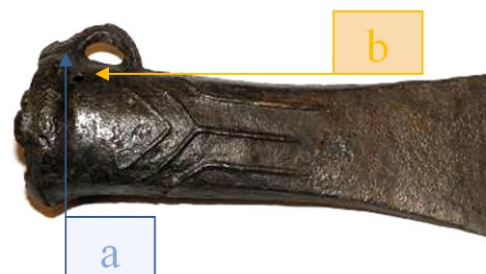
Fig. 5. Axe, visible remains of gating systems – marked in yellow (axe No. NG25)
