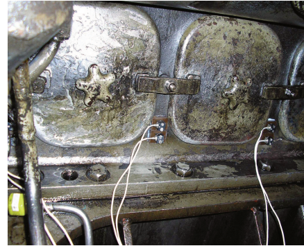
Fig. 2. Sensors mounted on an engine body
