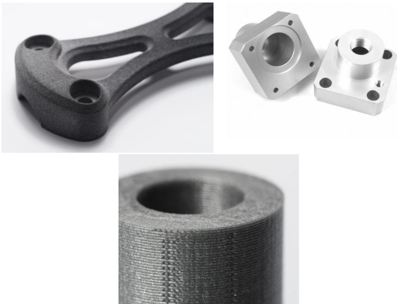
Fig. 2. Comparison of quality of the obtained external surfaces From left: CNC machining, FDM technology and MJF technology [4]
