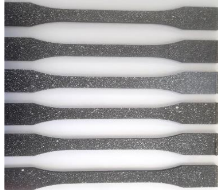
Fig. 4. Samples with a white pattern for testing with the use of digital image correlation (DIC) [8] [own study]
