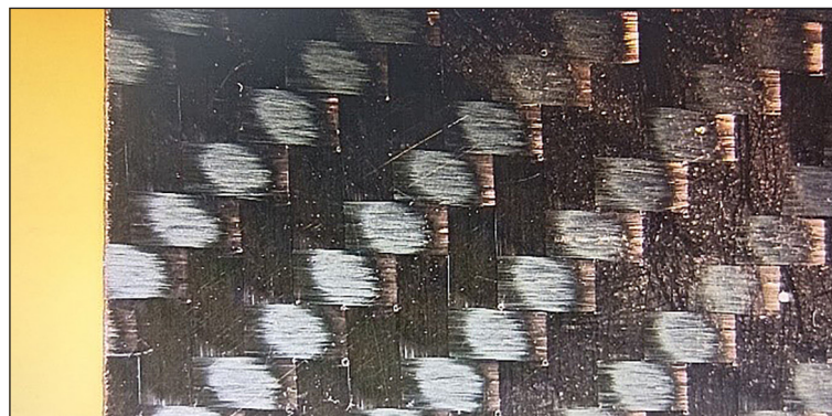
Fig. 5. Laminate surface made at a negative pressure of 0.7 bar
