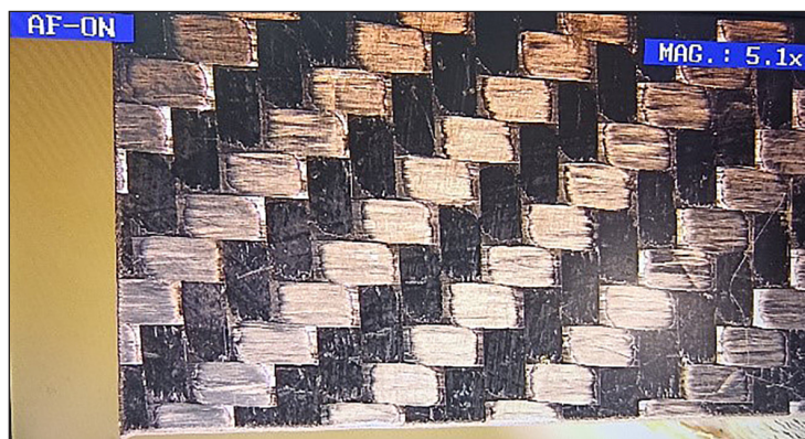
Fig. 7. Laminate surface made at a negative pressure of 1.0 bar
