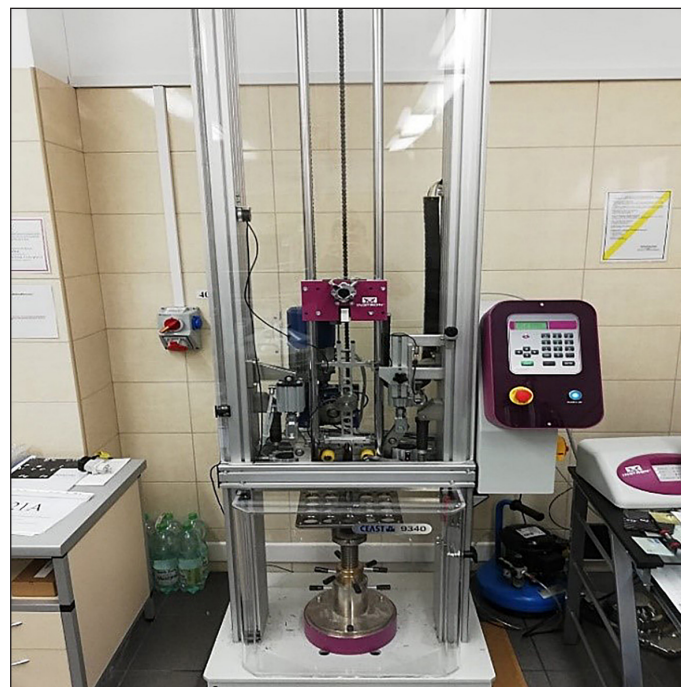
Fig. 15. Instron Ceast 9340 drop hammer
