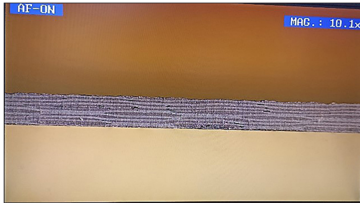
Fig. 6. Internal structure of a laminate made with a negative pressure of 0.7 bar
