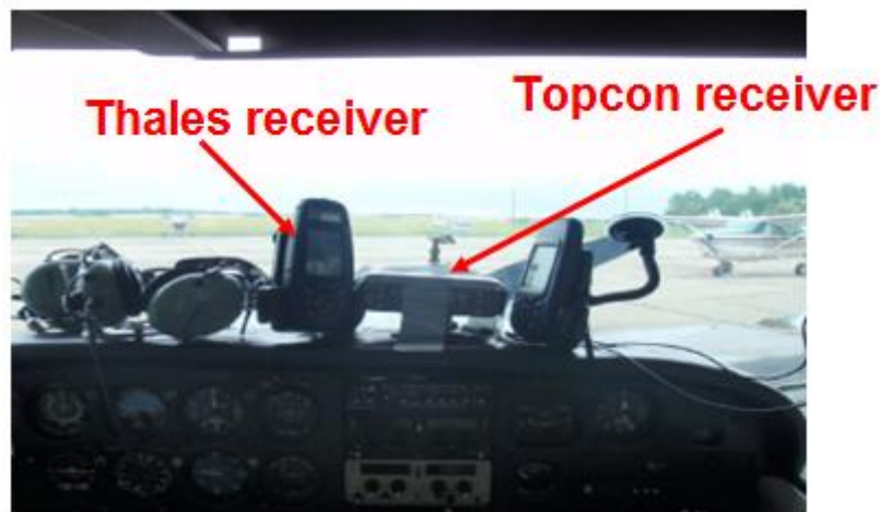
Fig. 1. Thales Mobile Mapper and Topcon HiperPro receivers onboard the Cessna 172 Source: scientific materials from the Institute of Navigation of MUA in Dęblin
