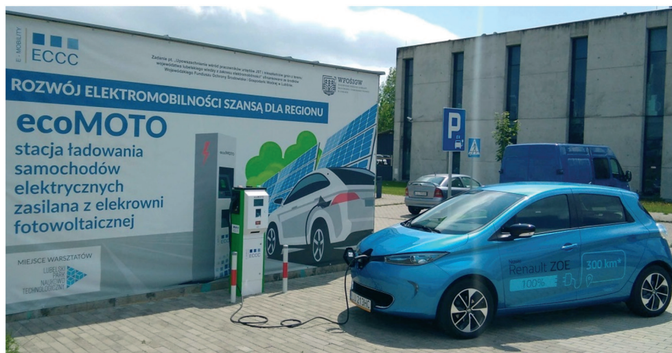
Fig. 1. Tested vehicle while charging from a 22 kW pole
