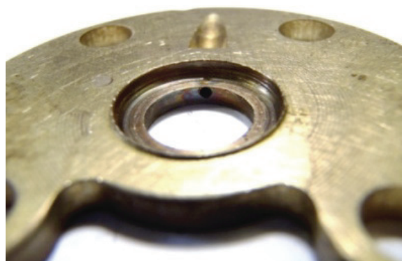
Fig. 11. View of bearing with hot tracks
