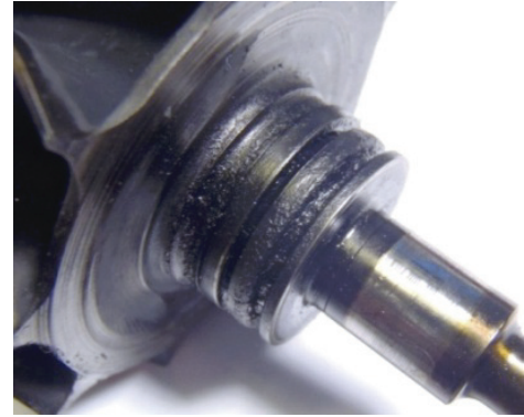
Fig. 5. View of rotor's shaft with ring seals becoming stuck in their grooves
