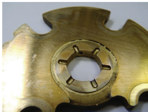
Fig. 3. View of scraped surface of bearing
