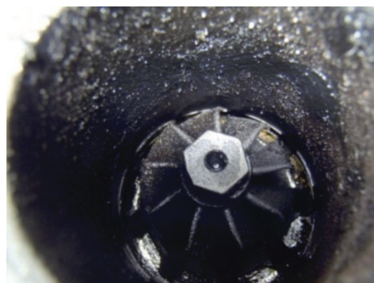
Fig. 10. View of turbine rotor with carbon depositing
