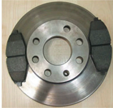
Fig. 4. Brake pad and brake disc for the Daewoo Lanos passenger car
