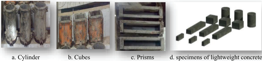
Fig. 4. Cylinder, Cubes, Prisms and specimens of lightweight concrete.
