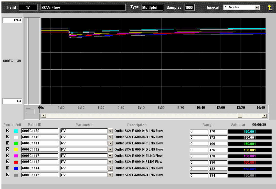
Fig. 4. Trend displays present values of process variables against the selected time axis
