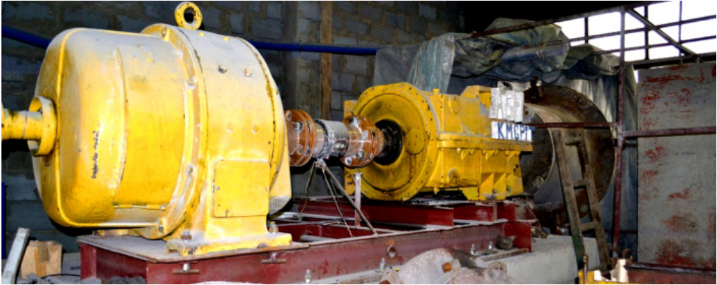
Fig. 8. Laboratory testing stand for examination of quality of tangential-rotary picks
