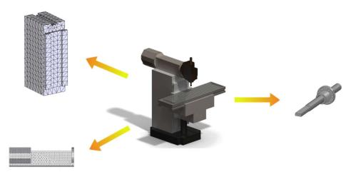
Fig. 1. The concept of modeling load-carrying systems in machines containing ball-screw mechanisms
