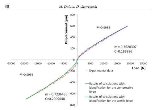
Fig. 6. Summary of computational and experimental characteristics and the identified parameters
