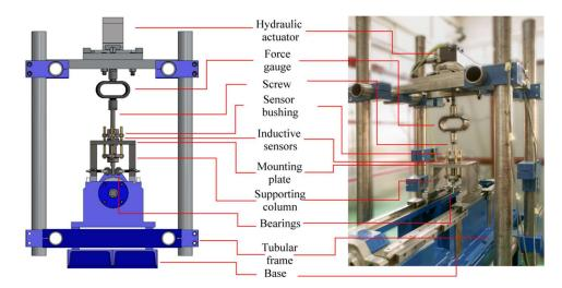
Fig. 3. The test bench for testing ball-screw mechanisms
