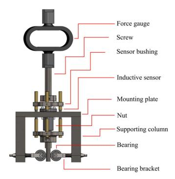
Fig. 3. Diagram of the test bench used to study the ball-screw mechanism
