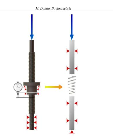
Fig. 5. Diagram of ball-screw mechanism modeling adopted in the identification process
