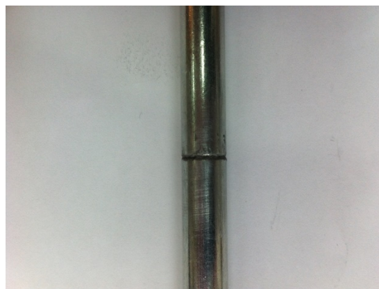
Fig. 10. Sample to be used for determining the shock energy
