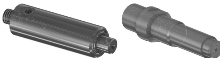
Fig. 1. Upper and lower injector body.
