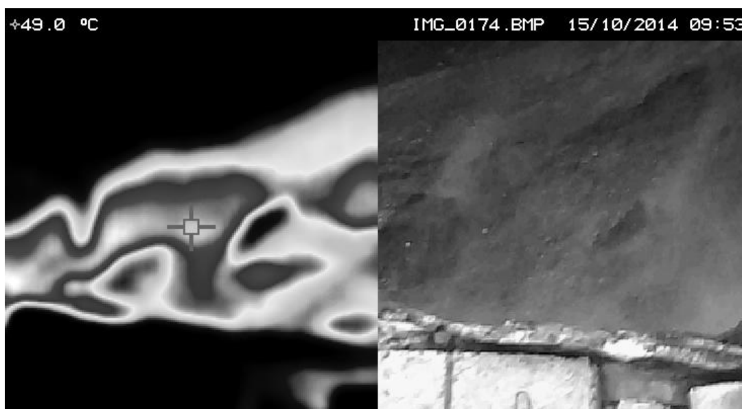
Fig. 1. Thermal image indicating the temperature range of the coal heap (Author: Bogdan Sobociński)
