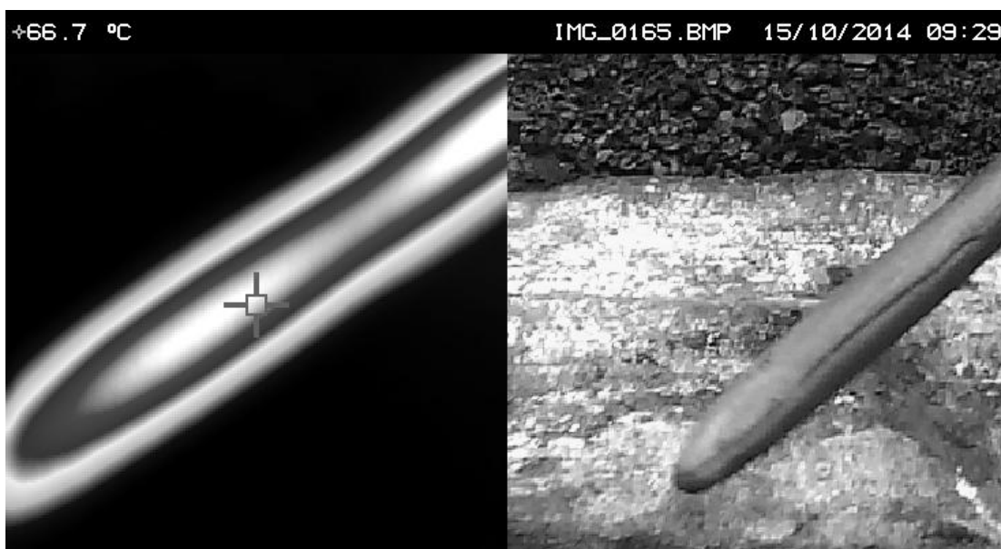
Fig. 3. Thermal image of a steel rod after immersion in the coal heap (Author: Bogdan Sobociński)
