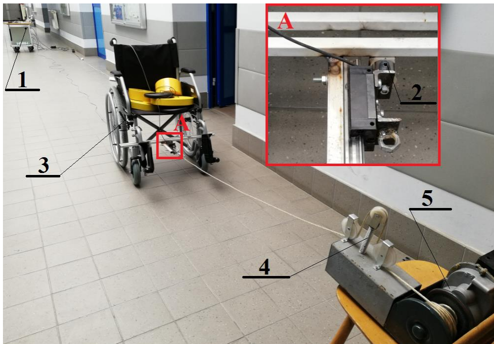
Fig. 3. Research on the rolling resistance coefficient in accordance with P.424484, where: 1 – monitoring-recording device, 2 – force measurement sensor, 3 – research object, 4 - rope tension adjusting system, 5 – drive system
