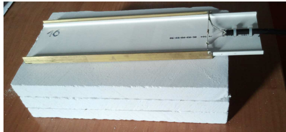
Fig. 4. Surface probe calibration for autoclaved calcium silicate
