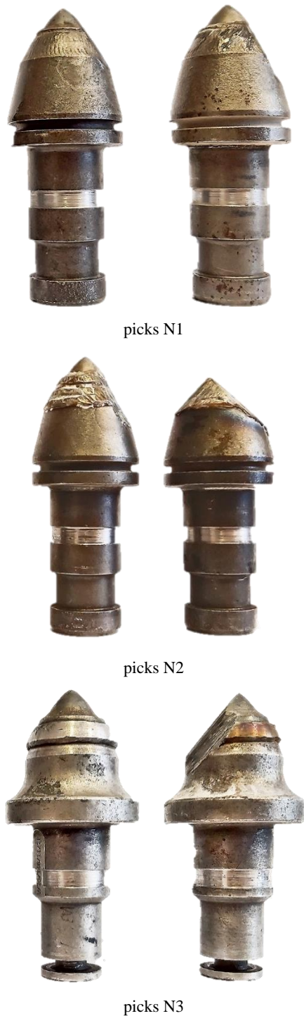
Fig. 8. View of selected picks after the tests prepared for measuring mass and volume
