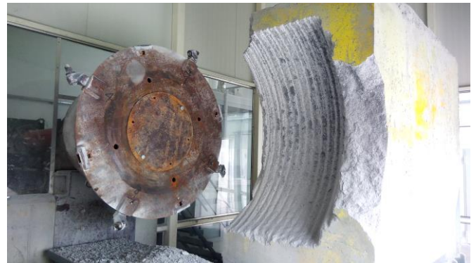
Fig. 2. A laboratory setup for studying the rock-cutting process using rotary milling or drilling head unit
