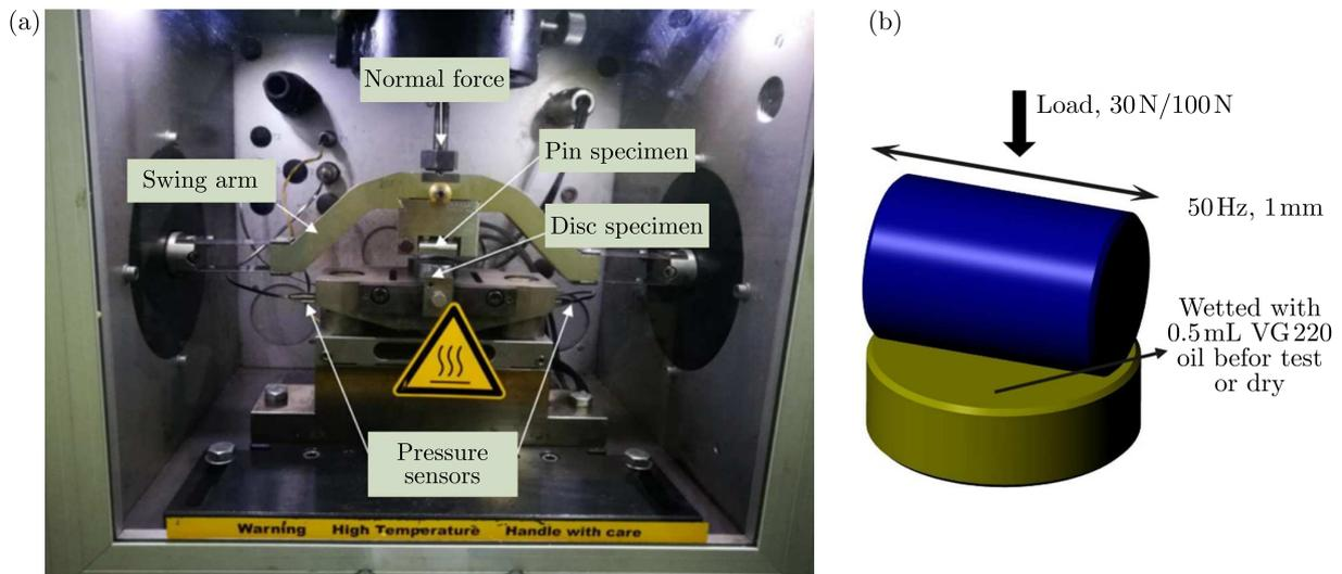
Fig. 3. (a) Test chamber of the SRV<sup>®</sup> IV test apparatus, (b) schematic representation of the pin-on-disc test specimens
