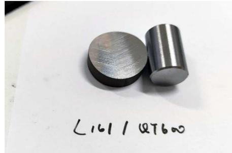
Fig. 1. Test specimens of pin and disc
