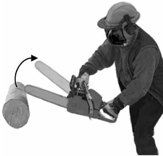
Figure 1. Chain saw kickback. Notes. a—kickback, b—hazardous contact of top part of guide bar with rigid object.
