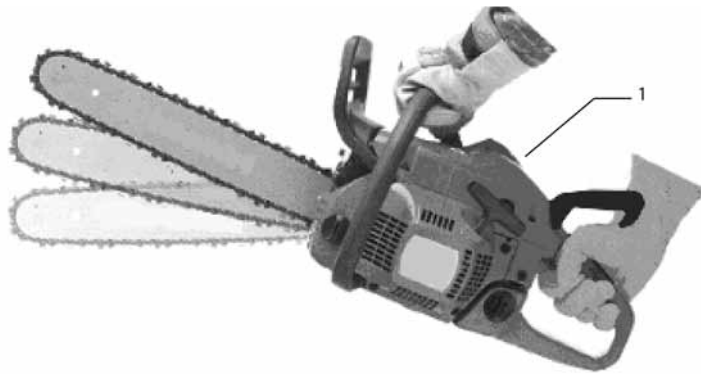
Figure 17. Another way of activating a chain brake. Notes. 1—additional lever for activating the chain brake.
