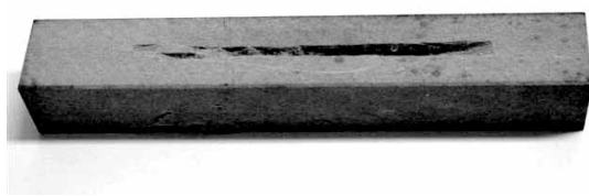
Figure 9. Wood kickback sample after contact with chain, a visible kerf.
