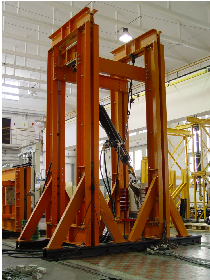
Fig. 3. Test set-up with the A400M engine cowl door hinge fitting specimen.
