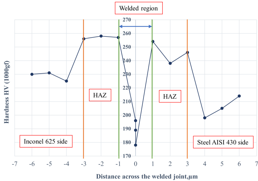
Figure 8. Distribution of hardness results in HV1 measured on transverse microsections of the welded joint
