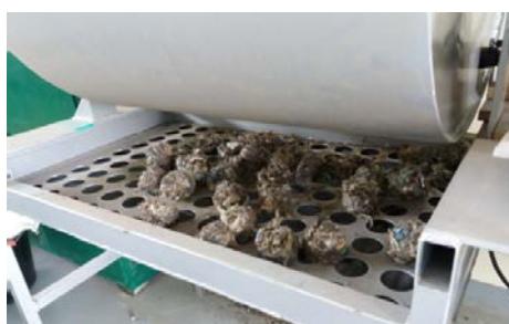
Figure 8. B type briquettes after the DU durability (image of a screen with meshes diameter of 35 mm under the drum tester).
