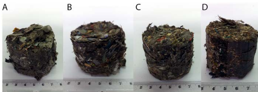
Figure 4. Briquettes obtained in the process of agglomeration in relation to biomass participation in the following composition: A – 0%, B – 10%, C – 25%, D – 50%
