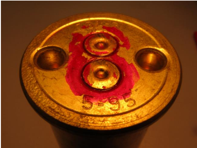
Fig. 3. Indentation marks from the firing pin on the primer cap bases of a cartridge
